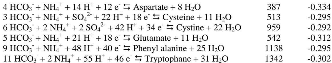
**Table 4. Gibbs energy change  $\Delta G_r^{0'}$  and equilibrium potential  $E_r^{0'}$  of specific half reactions with an organic electron acceptor. Calculated using the Growth Reference System (biochemical standard conditions: 1 atm, 298.15 K, 1 mol/L, pH 7). Data from Heijnen<sup>1</sup> unless otherwise indicated.**
