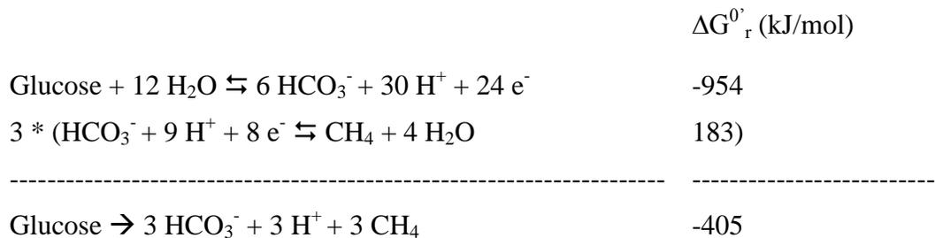
The Gibbs free energy of this reaction is less negative than the reaction with oxygen, implicating a less spontaneous process. Whenever oxygen is present, bacteria will use it as electron acceptor, since it is thermodynamically more favorable.
