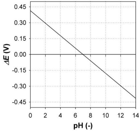
**Figure 1. Effect of pH on the equilibrium potential of half reactions that involve as many protons involved in the reaction as electrons (i.e.,  $\nu_H=n$ ) at 298.15 K.**
