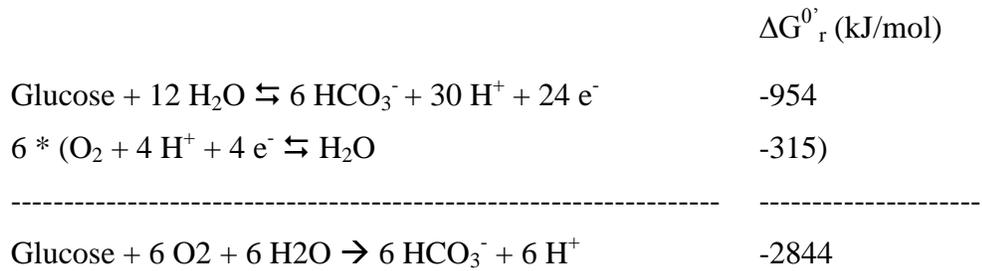
This reaction has a highly negative Gibbs free energy, implicating that this reaction is thermodynamically feasible for bacteria to perform.
